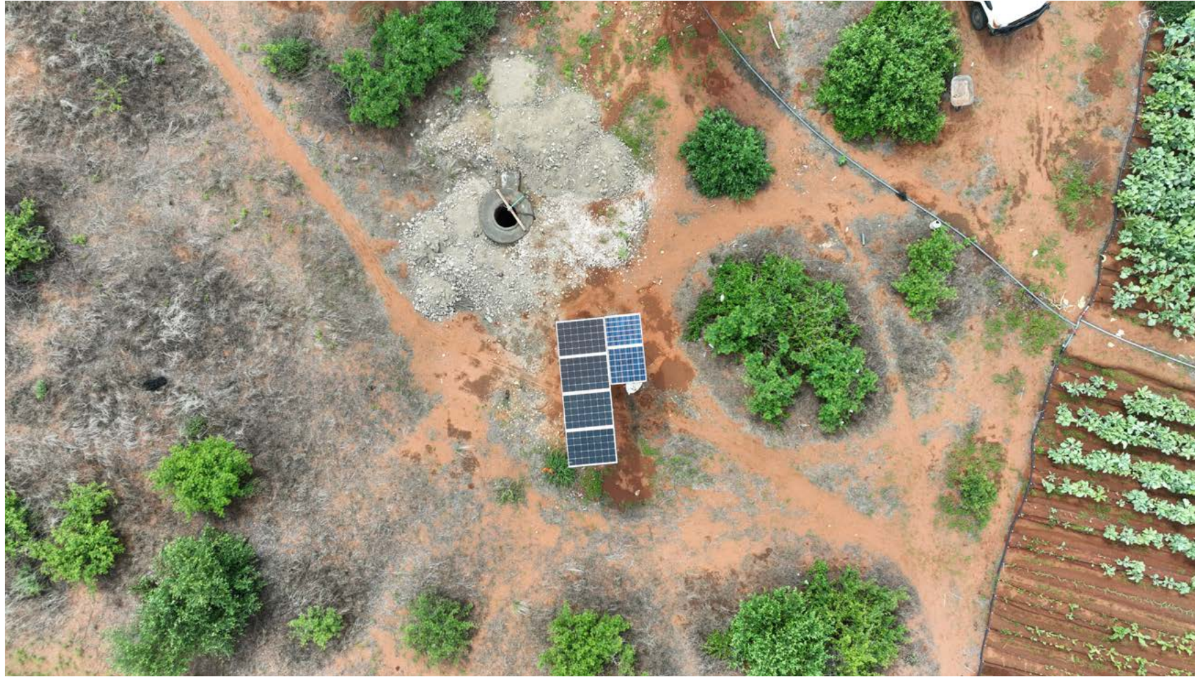
The project installs solar power to pump water from a nearby borehole to irrigate their farm.
