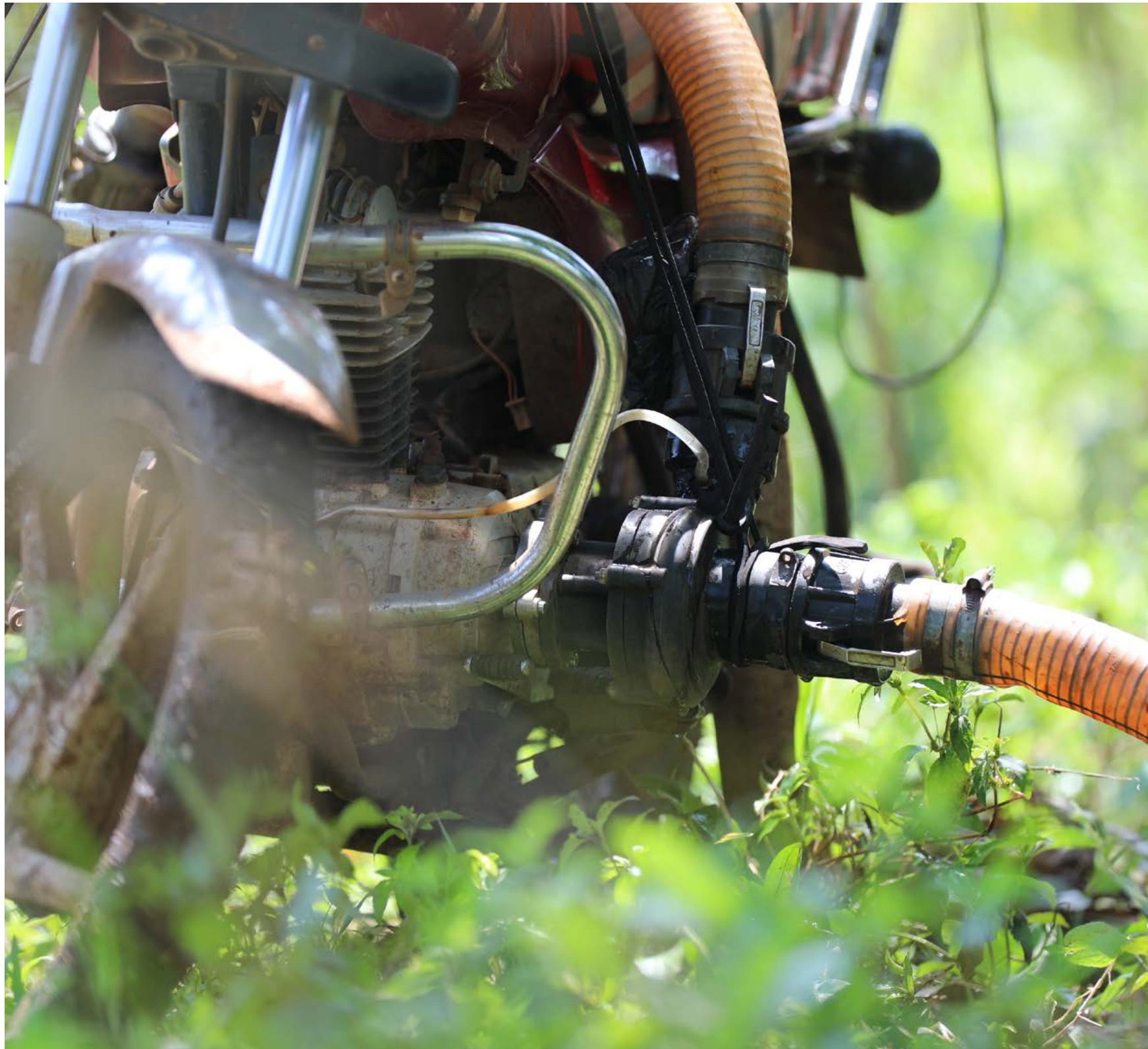
The mobile irrigation equipment is powered by a motorcycle engine to draw water from the source and pump it to a farm to irrigate crops.
